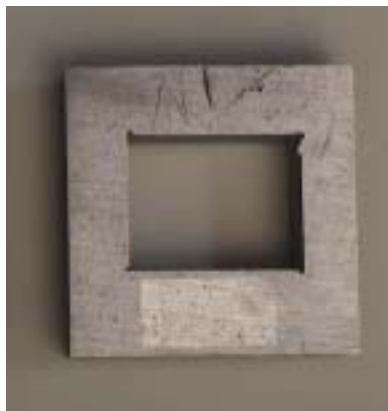
Figure 5. Inside corner damage caused by stream lag. The material in this image is 1" stainless steel, though this damage will occur on any material. The thicker the material the more significant the damage. Slowing down the cutting speed at corners will reduce the inside corner damage.
